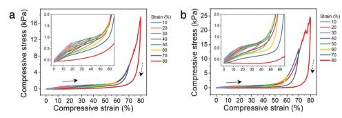
Fig. 5 Cyclic compression behavior of PANI hydrogels. Stress-strain curves during loading-unloading to various strains for (a) Kelvin lattice with 14% relative density, and (b) octet lattice with 16% relative density. Arrows and dashed arrows represent the loading and unloading directions, respectively. A loading and unloading rate of 100% min<sup>-1</sup> was used.
