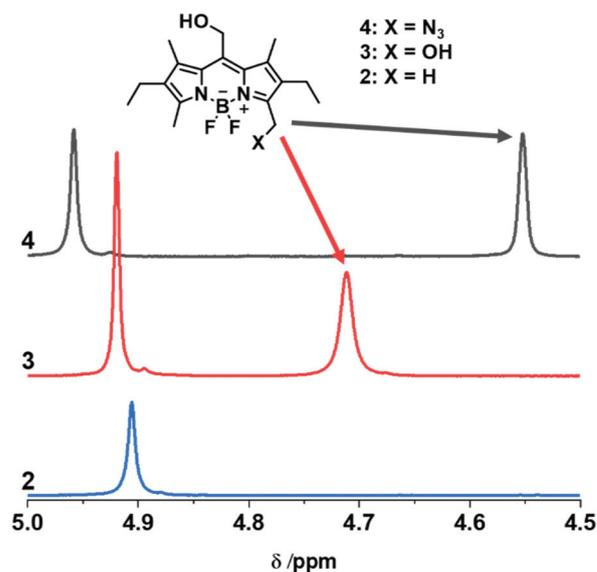
Fig. 3  $^1\text{H-NMR}$  spectra in  $\text{CDCl}_3$  of the hydrolysed BODIPY compound **2** (blue), the BODIPY-diol compound **3** (red) and the BODIPY-azide compound **4** (black) showing the proton signals arising upon the substitution at position 3 at 4.71 ppm and 4.55 ppm for the diol and the azide, respectively.
