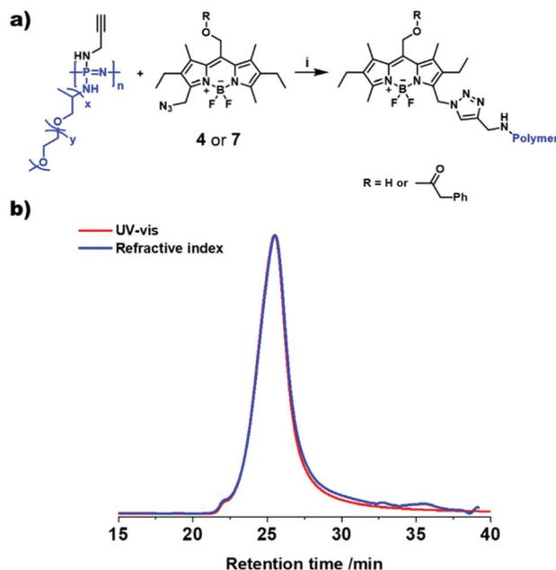
**Fig. 6** Loading of the BODIPY 4 or 7 onto the poly(organo)phosphazene. (a) Scheme of the reaction of BODIPY 4 or 7 with poly(organo)phosphazene. (b) SEC-traces of the UV-vis (540 nm) and the refractive index detectors, showing an overlap of the signals and indicating a successful loading of the BODIPY compound 7 onto the poly(organo)phosphazene carrier. (i)  $\text{CuSO}_4 \cdot 5\text{H}_2\text{O}$ , (+)-L-Na ascorbate,  $\text{DCM}/\text{H}_2\text{O}$ .
