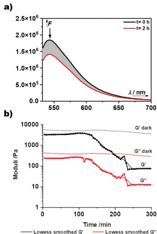
**Fig. 4** Kinetic studies of the photodegradation of the BODIPY-diol containing hydrogel. (a) Decrease of the fluorescence intensity upon irradiation of the BODIPY-hydrogel at 510 nm for 2 h. (b) Photorheology measurements of the BODIPY-hydrogel and the stability of the gel in the dark. Light on after 2 min.
