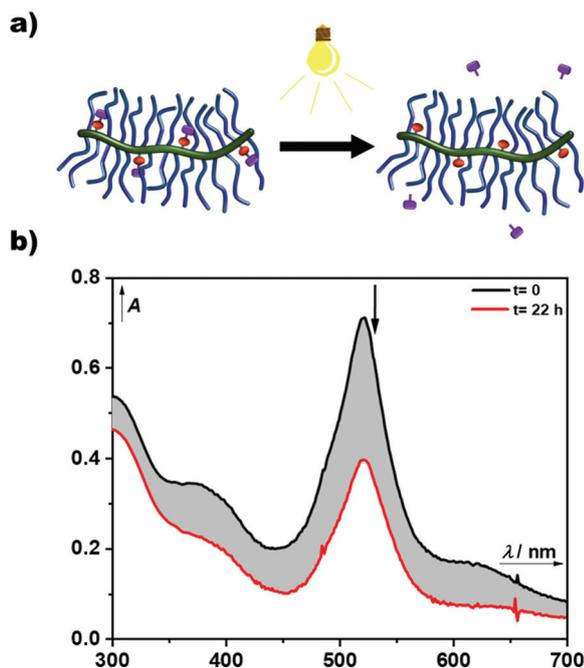
**Fig. 7** Photoreaction of the BODIPY decorated poly(organo)phosphazene. (a) Cartoon visualising the light-stimulus controlled release of conjugated phenylacetic acid from the BODIPY decorated polymer carrier. (b) Kinetic study of the photodegradation of the BODIPY decorated poly(organo)phosphazene in MeOH upon 505 nm LED irradiation for the indicated time.
