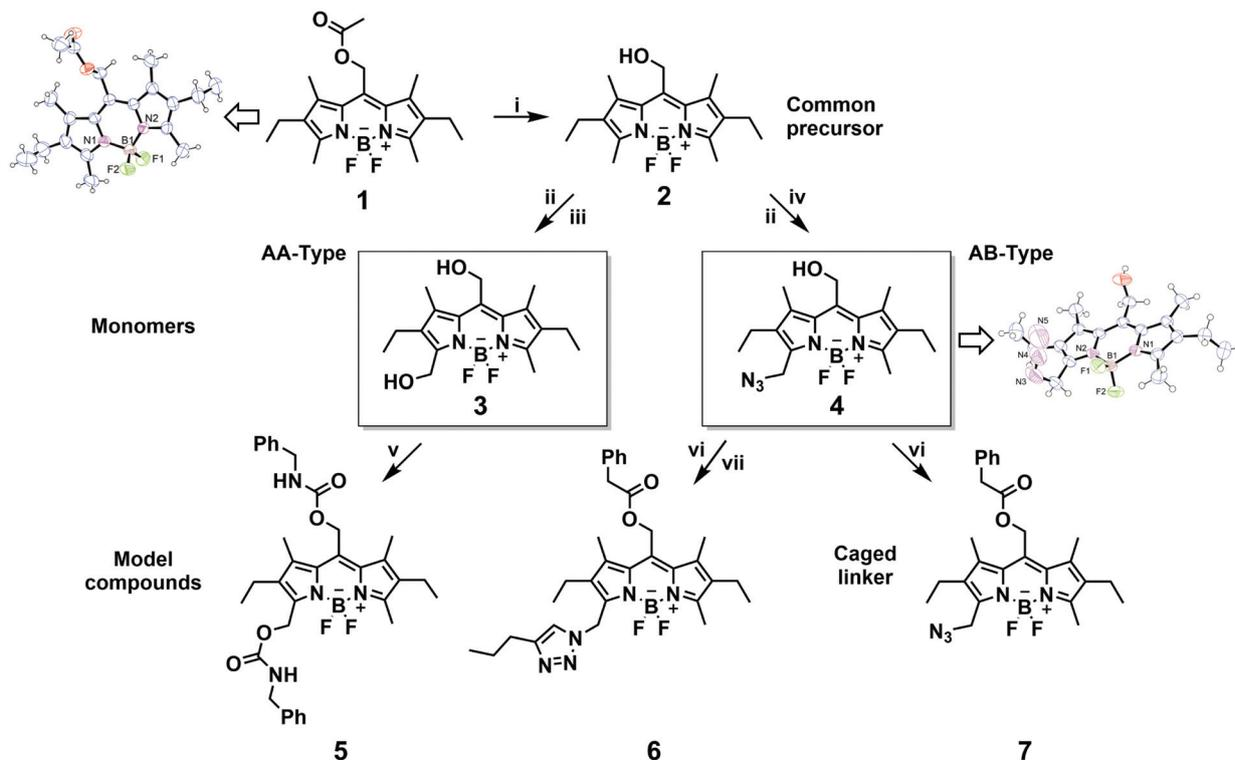
**Scheme 1** Synthesis pathway towards bifunctional and hetero-bifunctional BODIPY monomers **3** and **4** and the synthesis of their respective small-molecular model compounds **5–7**. (i) NaOH, DCM/MeOH, H<sub>2</sub>O; (ii) NBS, DCM; (iii) H<sub>2</sub>O/DCM; (iv) NaN<sub>3</sub>, DCM/DMF; (v) benzyl isocyanate, toluene; (vi) phenylacetic acid, DCC, DMAP, DCM; (vii) pentynes, CuSO<sub>4</sub>·5H<sub>2</sub>O, (+)-L-Na ascorbate, DCM/H<sub>2</sub>O.
