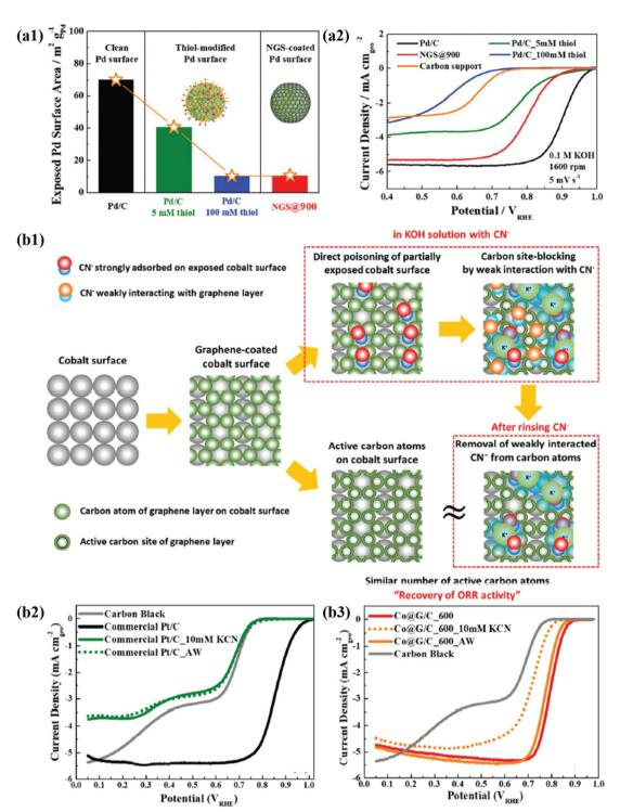
Fig. 7 (a1) The exposed Pd surface area of Pd@C. (a2) ORR polarization curves of Pd/C, Pd/C-5 mM thiol, NGS@900, Pd/C\_100 mM thiol, and carbon support, reproduced with permission from ref. 48, RSC publications copyright 2019. (b1) Schematic illustration of the mechanism for CN effect on Co@G/C. (b2) ORR polarization curves of commercial Pt/C. (b3) Co@G/C in 0.1 M KOH with 10 mM KCN and after cleaning in pure 0.1 M KOH, reproduced with permission from ref. 47, RSC publications copyright 2019.
