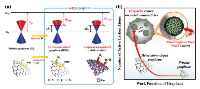
Fig. 2 Schematic illustration of the electronic effects between the carbon shell and metal nanoparticles (a) Design concept to modify the work function of the carbon shell *via* Co encapsulation, adapted from ref. 47 with permission from RSC publications, copyright 2019. (b) Advantages of carbon shell encapsulated Pd nanoparticle catalysts, adapted from ref. 48 with permission from RSC publications, copyright 2019.
