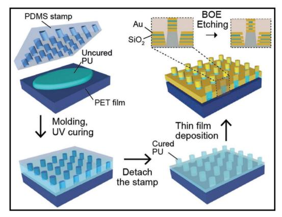
Fig. 8 Schematic of the preparation of nanolaminated SERS substrate with three insulator layers. Reproduced with permission. <sup>121</sup> Copyright 2019, WILEY-VCH Verlag GmbH & Co. KGaA, Weinheim.
