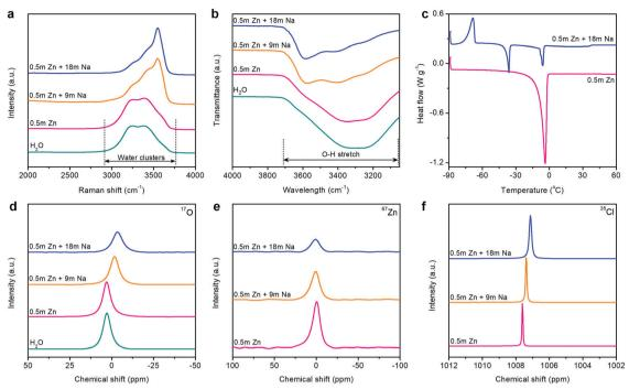
Fig. 2 Spectroscopic characterizations of the electrolytes. (a) Raman spectra, (b) FT-IR spectra, (c) DSC profiles, (d) <sup>17</sup>O (water) NMR spectra, (e) <sup>67</sup>Zn NMR spectra, and (f) <sup>35</sup>Cl NMR spectra.
