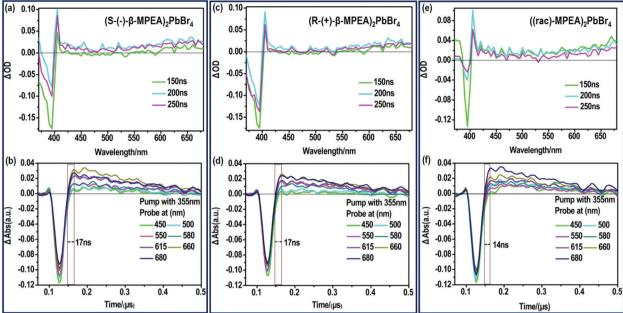
Fig. 3 ns-TA spectra of (a) (S-β-MPEA)<sub>2</sub>PbBr<sub>4</sub>, (c) (R-β-MPEA)<sub>2</sub>PbBr<sub>4</sub>, (e) ((rac)-MPEA)<sub>2</sub>PbBr<sub>4</sub> films upon excitation at 355 nm. TA onsets of (b)  $(S-\beta-MPEA)_2PbBr_4$  (d)  $(R-\beta-MPEA)_2PbBr_4$ , (f)  $((rac)-MPEA)_2PbBr_4$  films probed at different wavelength.
