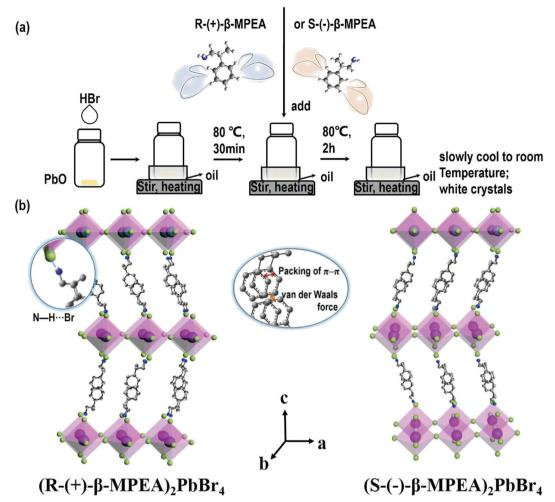
Scheme 1 (a) The schematic experimental operation diagram. (b) The structural illustration of crystals of  $(R-(+)-\beta-$  and  $S-(-)-\beta-$  MPEA)<sub>2</sub>PbBr<sub>4</sub> (yellowgreen ball = bromide atom, sky-blue ball = lead atom, gray ball = carbon atom, deep-blue ball = nitrogen atom, and pink-white ball = hydrogen atom).
