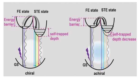
Fig. 5 Diagram of luminescence processes in the as-formed perovskite crystals. (GS: ground state, FE state: free-exciton state, STE state: self-trapped
