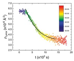
Fig. 5  $\,$  Time evolution of the  $\rho_{\rm t_{\rm Drox}}$  parameter obtained from the analysis of the TTR-NR data measured according to the constant temperature steps profile. Values obtained at different temperatures are labelled with different colors in the graph. The model of the time-dependent kinetic evolution (egn (5)) is plotted as full line for the temperature range analysed.
