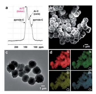
Fig. 2 (a)  $^{13}$ C solid-state NMR spectrum of PV-COF with peaks assigned to relevant carbon atoms; (b) SEM image of PV-COF shows spherical particles with an average size of 1.4  $\mu$ m; (c) TEM image of PV-COF; (d) elemental mapping of Zn-PV-COF showing an even distribution of constituent elements (C, N, Cl and Zn).
