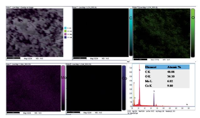
Fig. 4 Elemental analysis of the synthesized nanomaterial using energy dispersive X-ray spectroscopy.
