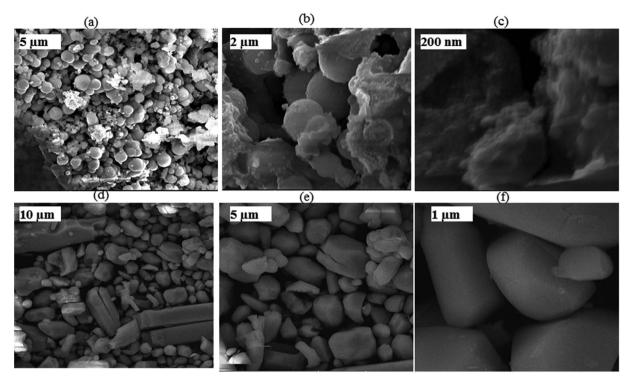
Fig. 6 (a-c) FE-SEM images of the organic template-assisted  $CoMoO_4$  at different magnifications. (d-f) FE-SEM images of the controlled sample (ethylene glycol assisted  $CoMoO_4$ ) at different magnifications.
