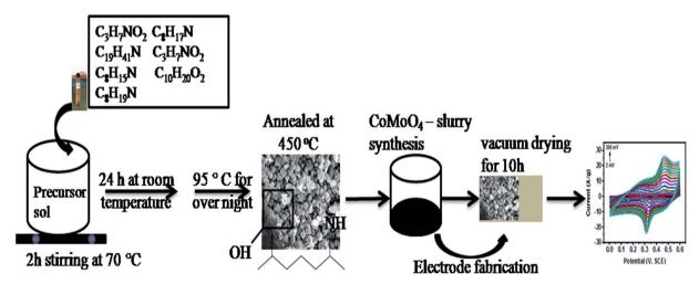
Fig. 1 Schematic diagram of the modified hydrothermal method via organic compounds to synthesize CoMoO<sub>4</sub> for fabrication of the electrode.
