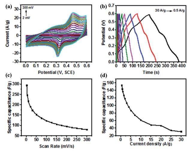
Fig. 8 (a) Cyclic voltammograms of the  $CoMoO_4$  electrode at various scan rates. (b) Galvanostatic charge–discharge characteristics of  $CoMoO_4$  at various current densities. (c) Variation of the specific capacitance as a function of the scan rate, and (d) variation of the specific capacitance as a function of the applied current density.
