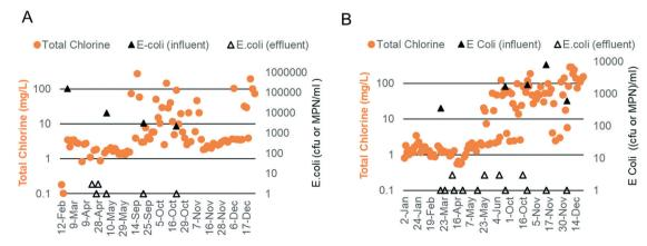
Fig. 6 *E. coli* levels in the blackwater and treated water *versus* total chlorine at sites A and B indicated disinfection. Bacterial counts in the treated water were measured by plate counting (1 CFU per ml resolution) and MPN methods (3 MPN per ml resolution).
