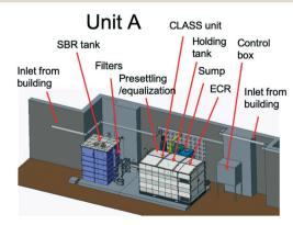
Fig. 2 Layout of the installation at site A with a SBR biological pretreatment system.
