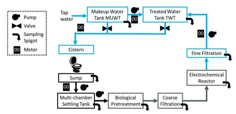
Fig. 1 Flow diagram of the CLASS.
