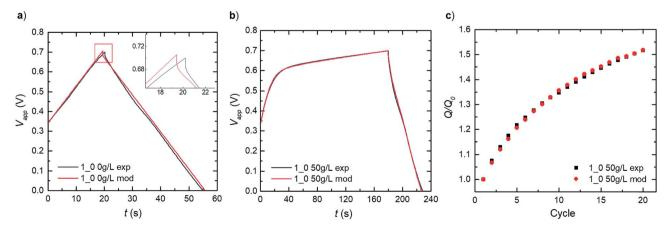
Fig. 3 Comparison of model and experimental results for galvanostatic charge-discharge at 566  $\mu$ A (2 A g<sup>-1</sup>): (a) PEDOT:PSS + NFC without preloaded LS (1\_0) and 0 g L<sup>-1</sup> LS in electrolyte (no changes with cycling). (b) Cycle 1 of 1\_0 electrode with initial 50 g L<sup>-1</sup> LS dissolved in bulk electrolyte. (c) Relative discharge capacity recorded for 20 cycles following (b).  $L_F$  is 52  $\mu$ m in both (a) and (b).
