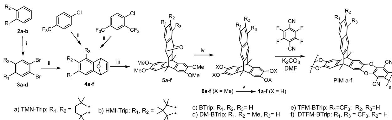
Fig. 1 Structure and synthesis of the benzotriptycene PIMs. Reagents and conditions: i.  $Br_2$ , Fe, DCM, rt, 3 h; ii. *n*-BuLi, furan, THF,  $-78^\circ C$ , 1.5 h; iii. 9,10-Dimethyl-2,3,6,7-tetramethoxyanthracene, DMF, 250  $^\circ C$ , 7 bar, 2 h, microwave irradiation, iv. TFA or  $MeSO_4H$ , rt, 24 h; v.  $BBr_3$ , DCM. (See ESI† for details).
