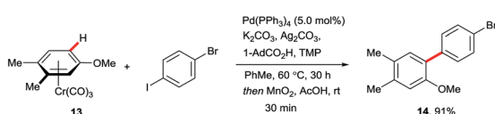
Scheme 2 C-H functionalisations exploiting the reactivity of \pi -Cr complexes.
