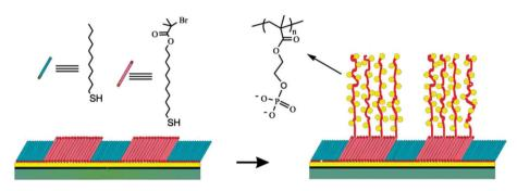
Fig. 23 Procedure for patterned polymer brush formation on gold substrates. Polymer brush growth from initiator modified areas (Copyright 2005, The Royal Society of Chemistry, modified from ref. 392).
