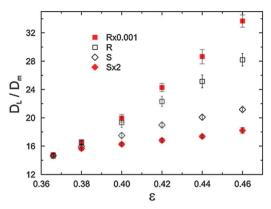
Fig. 22 Asymptotic longitudinal dispersion coefficients  $(D_1)$  normalized by the molecular diffusivity in bulk solution  $(D_m)$  at a particle Péclet number of Pe = 50, i.e., in the advection-dominated transport regime, for the different sphere packing types as a function of bed porosity. Error bars indicate 95% confidence intervals. Reprinted from Khirevich et al.<sup>22</sup> Copyright 2010 with permission from Elsevier
