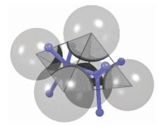
Fig. 10 Delaunay tessellation for a set of spheres. The tetrahedron represents the pore that is enclosed by the four shown spheres. Blue bars indicate the edges of the Voronoi cell for the same set. Reprinted from Charevre et al. 148 Copyright 2012, with permission from Springer.
