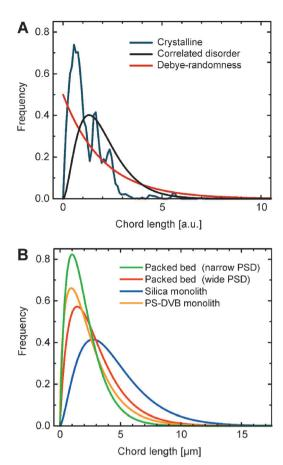
Fig. 17 (A) Characteristic CLDs for materials with different types of (dis)-order. (B) Comparison between structurally differing materials exhibiting correlated disorder: sphere packings obtained using a narrow or wide particle size distribution (PSD), *i.e.*, with  $\sim$ 3% or  $\sim$ 18% relative standard deviation of the PSD, a silica monolith, and a poly(styrene–divinylbenzene) (PS–DVB) monolith.
