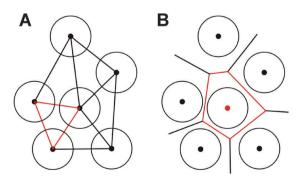
Fig. 9 Generation of Delaunay tessellation (A) and Voronoi tessellation (B) for 2D disks of the same size. Reprinted from Khirevich et al.<sup>23</sup> Copyright 2011, with permission from Elsevier.
