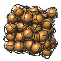
Fig. 11 Voronoi tessellation for a set of randomly arranged, identical spheres. Reprinted with permission from Schröder-Turk et al. 149 Copyright 2013, American Institute of Physics.
