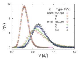
**Fig. 14** Distribution P(V) of normalized Voronoi cell volumes V for computer-generated random packings of monosized spheres at bed porosities of  $\varepsilon = 0.366$  and 0.46 as a function of packing type. Reproduced from Khirevich *et al.*<sup>23</sup> Copyright 2011, with permission from Elsevier.
