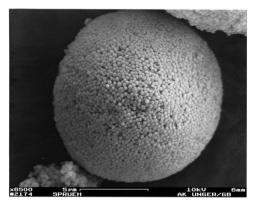
Scanning electron micrograph of a micrometer-sized bead formed from nonporous spherical silica nanoparticles through a spray-drying process. Scale bar, 5 µm. The original particles forming the interstitial mesopore space in the final bead can be clearly identified
