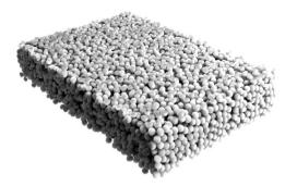
Fig. 6 Reconstructed bed of 2.6 μm spherical core-shell particles packed into a 100 μm inner-diameter cylindrical fused-silica capillary. The reconstruction covers a capillary segment of 100  $\mu$ m (entire capillary diameter)  $\times$ 58  $\mu m$  (along the column axis) imes 15  $\mu m$ . The imaging of the packing microstructure is based on confocal laser scanning microscopy, realized by adapting a refractive index matching approach. 108
