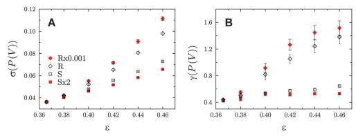
Fig. 15 Standard deviation (A) and skewness (B) of Voronoi volume distributions for the different packing types as a function of bed porosity. The corresponding distributions for  $\varepsilon = 0.366$  and 0.46 are shown in Fig. 14. Reproduced from Khirevich *et al.*<sup>23</sup> Copyright 2011, with permission from Elsevier.
