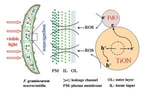
Fig. 7 Photocatalytic disinfection mechanism of TiON/PdO photocatalyst on Fusarium graminearum macroconidia under visible light irradiation. Reproduced with permission from ref. 157, copyright (2013) American Chemical Society.
