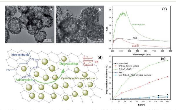
Fig. 3 The HRTEM images of the prepared ZnSnO<sub>3</sub> hollow nanosphere (a) and ZnSnO<sub>3</sub>/RGO nanocomposite (b). (c) The UV-Vis absorption spectra of the RGO, pure  $ZnSnO_3$  hollow nanosphere and  $ZnSnO_3/RGO$  nanocomposite. The speculated illustration (d) and degradation efficiencies (e) of the metronidazole wastewater by ZnSnO3 hollow nanosphere and ZnSnO3/RGO nanocomposite photocatalysts under visible light irradiation. Reproduced with permission from ref. 33.
