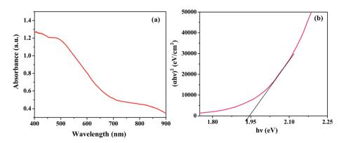
Fig. 3 (a) Diffuse reflectance spectra and (b)  $(\alpha h \nu)^2 vs. h \nu$  plot of ZnFe<sub>2</sub>O<sub>4</sub> annealed at 400 °C.
