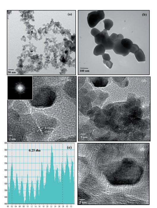
Fig. 1 TEM images of  $CuFe_2O_4$  annealed at (a)  $400\,^{\circ}C$  and (b)  $1000\,^{\circ}C$ , HRTEM images of the  $CuFe_2O_4$  nanoparticles at (c) magnification of 2 nm (inset shows the FFT of  $CuFe_2O_4$ ) and (d) magnification of 5 nm. (e) Frame profile for the average fringe width. (f) Reconstructed image after filtering the FFT pattern from HRTEM.
