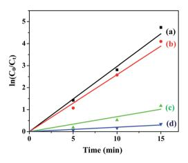
Fig. 7 Photodegradation kinetics of MB in the presence of (a)  $CuFe_2O_4$ , (b)  $ZnFe_2O_4$ , (c)  $NiFe_2O_4$  and (d)  $CoFe_2O_4$  under optimum conditions.
