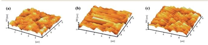
Fig. 6 3D surface AFM images of the membranes with different HMO/PES ratios, (a) PES, (b) PES/HMO-1 and (c) PES/HMO-2.
