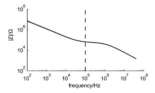
**Fig. 6** The measured frequency behaviour of the microfluidic chip. The black line in the graph is the average of 50 measurements obtained with the impedance/gainphase analyzer. The dashed line indicates the measurement frequency used during all subsequent experiments.
