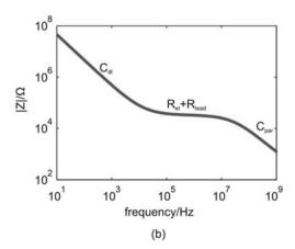
Fig. 1 (a) The simplified equivalent circuit model of the microfluidic device without a particle or cell in the channel. The interface between the two planar electrodes and the electrolyte is represented by the double layer capacitance ( $C_{dl}$ ).  $R_{el}$  is the electrolyte resistance,  $R_{lead}$  the lead resistance and  $C_{par}$  is the parasitic capacitance. (b) Typical frequency response of the real electrical impedance of the equivalent circuit model.
