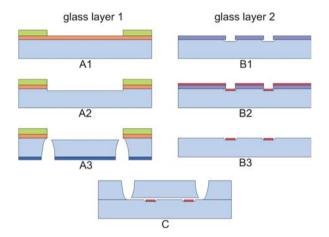
Fig. 3 Schematic diagram of the fabrication process. Glass layer 1 is firstly sputtered with Cr and Au, which is subsequently coated with a resist. After several lithography steps (A1), the microchannel is made by isotropically etching (A2). Access holes were powder blasted (A3). On glass layer 2 first a lithography step is done (B1). Subsequently platinum is sputtered (B2) and the electrodes are created by lift-off (B3). Bonding of the two glass wafers (C) creates the chip.
