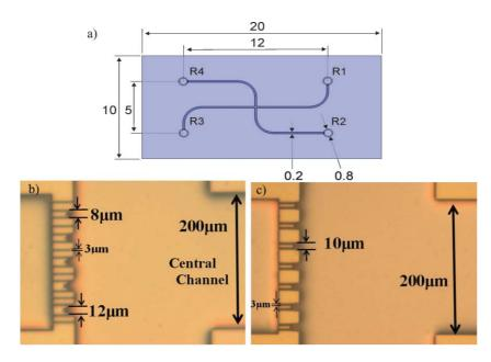
Fig. 1 (a) Drawing of the microfluidic chip with dimensions in mm. Photographs of the trapping sites, (b) layout 1 and (c) layout 2, in the microfluidic chip design.
