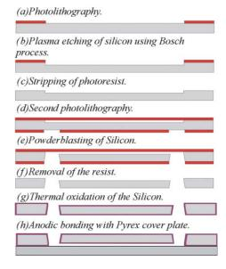
Fig. 3 Schematic of the fabrication process.
