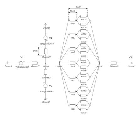
Fig. 4 Equivalent electrical circuit of the cell trapping device (layout 2) using 20-Sim (Control Lab Products B. V., Enschede).
