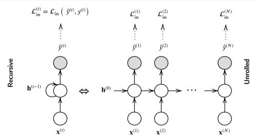
Fig. 6 A recurrent neural network in its recursive form (left) and unrolled form (right), where  $\mathscr{L}_{\text{in}}^{(t)}$  denotes the in-sample loss at the t-th time step. In practice, the initial hidden state of a RNN,  $\mathbf{h}^{(0)}$ , is usually set to the zero vector, and the expected loss is usually computed as the average loss over all time steps:  $\frac{1}{N} \sum_{t=1}^{N} \mathscr{L}_{\text{in}}^{(t)}$ .
