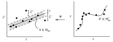
Fig. 3 Depiction of a nonlinear hypothesis in  $\mathcal{X}$ -space designed by transforming the problem into feature space  $\mathcal{Z}$  through a non-linear transform  $\Psi$ , and using SVM (a linear method) in the feature space.
