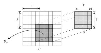
Fig. 5 Convolution visualized as sliding a filter (A) over an input (U).
