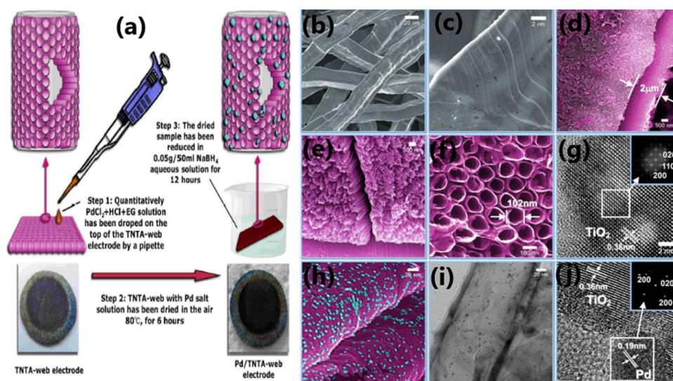
Fig. 24 (a) Synthesis of Pd/TNTA-web (3D TiO<sub>2</sub> nanotube array). Scanning electron microscopy (SEM) images of the pristine titanium-web substrate (b) and (c) and TiO<sub>2</sub> nanotubes arrays on the web (d), (e) and (f). HR-TEM image of a nanotube (g), SEM image (h), TEM image (i) and HRTEM image (j) of the TNTA-web with 0.1 mg cm<sup>-2</sup> Pd (0.26 wt%). Reproduced with permission from ref. 205. Copyright ©2018, the Royal Society of Chemistry.
