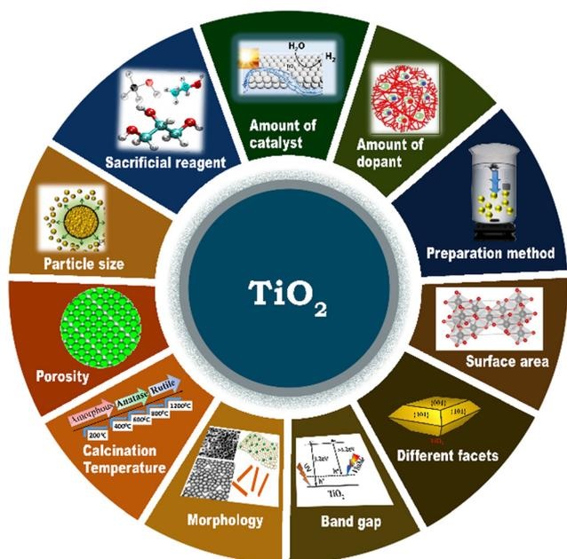
Fig. 15 Schematic representation of the various factors that determine the photocatalytic hydrogen evolution activity of TiO<sub>2</sub>-based photocatalysts.
