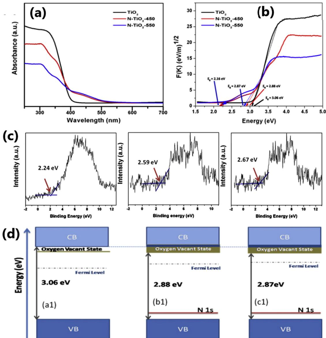
Fig. 7 (a) UV-vis absorbance spectra and (b) Tauc plot obtained from the reflectance spectra and (c) valence band edge analysis of TiO<sub>2</sub>, N-TiO<sub>2</sub>-450, N-TiO<sub>2</sub>-550. (d) Proposed band diagrams of TiO<sub>2</sub> and N-doped TiO<sub>2</sub> catalysts. Reproduced with permission from ref. 115. Copyright©2016, Elsevier Ltd.
