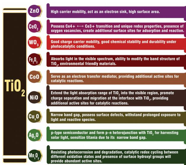
Fig. 9 Schematic representation of various metal oxides used for improving the photocatalytic hydrogen evolution activity of TiO<sub>2</sub>.
