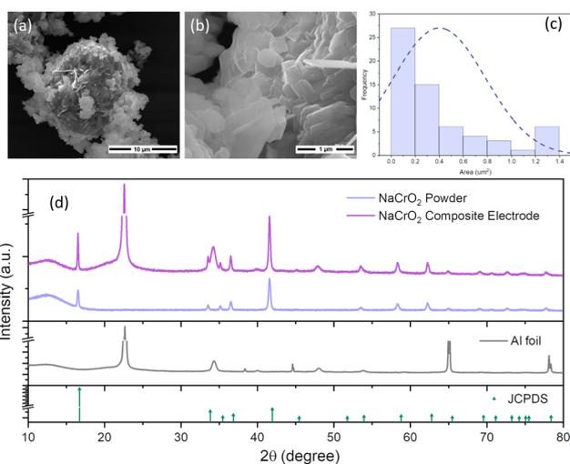
**Fig. 1** (a) and (b) SEM images of pristine NaCrO<sub>2</sub> powder, (c) particle size distribution of NaCrO<sub>2</sub> powder and (d) X-ray diffraction pattern of pristine NaCrO<sub>2</sub>, a composite electrode of NaCrO<sub>2</sub>, aluminium foil (utilized as a current collector for composite electrode) and the JCPDS file of NaCrO<sub>2</sub> for reference.
