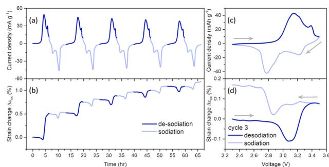
**Fig. 2** (a) Current density and (b) strain change in NaCrO<sub>2</sub> cathodes with respect to time during the cyclic voltammetry at 50  $\mu\text{V s}^{-1}$  rate between 2.3 to 3.5 V. (c) Current density and (d) strain change with respect to voltage during 3rd cycle, the strain is set to zero at the beginning of the 3rd cycle.
