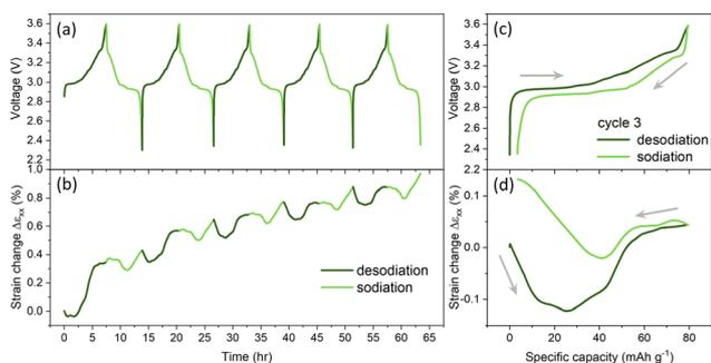
**Fig. 3** (a) Voltage profile and (b) strain evolution of NaCrO<sub>2</sub> cathode versus time during cycling at C/25 between 2.3–3.6 V for five cycles. (c) Voltage and (d) strain change is plotted against specific capacity in the third cycle and strain was set to zero at the beginning of third cycle for better comparison.
