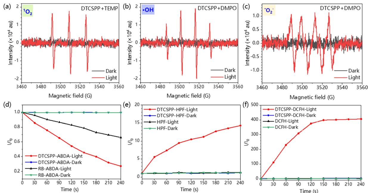
**Fig. 3** EPR spectra of (a)  $^1\text{O}_2$  trapped by TEMP, (b)  $\cdot\text{OH}$ , and (c)  $\cdot\text{O}_2^-$  trapped by DMPO and with and without laser irradiation. The plot of relative PL intensity of (d) ABDA (for  $^1\text{O}_2$  detection), (e) HPF (for  $\cdot\text{OH}$  detection), and (f) DCFH in the presence of  $1\ \mu\text{M}$  DTCSP or Rose Bengal (RB) upon white light irradiation for 1 min.
