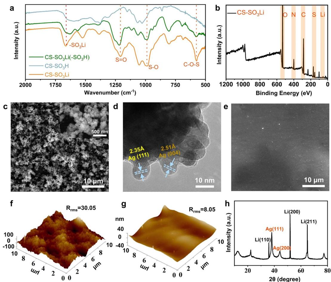
Fig. 2 Chemical and morphological analysis of LCS and nano-Ag modifications: (a) FTIR spectra of CS-SO<sub>3</sub>H (blue line), CS-SO<sub>3</sub>Li (green line) and AgLi-CS-SO<sub>3</sub>Li (orange line) samples; (b) XPS spectra of LCS; (c) SEM and (d) TEM micrographs of nano-Ag modified lithium anodes; (e) SEM images of LCS-Ag coated anodes; AFM topographies with (f) nano-Ag and (g) LCS-Ag coatings; (h) XRD patterns of LCS-Ag modified anode.
