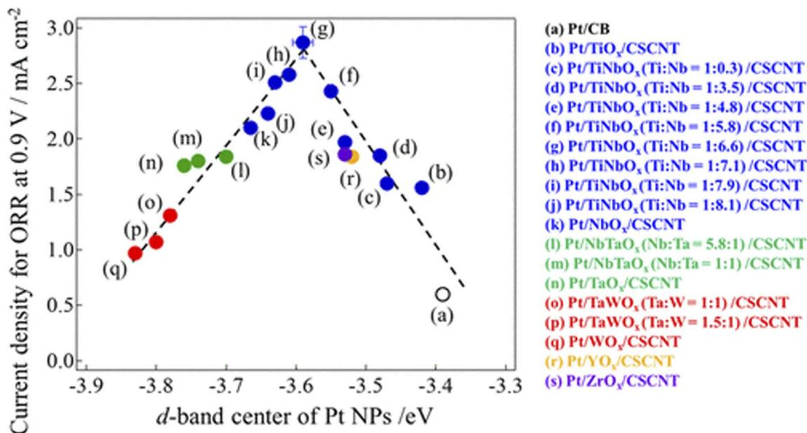
Fig. 7 Current density for the oxygen reduction reaction (ORR) at 0.9 V versus the d-band center of Pt nanoparticle curve. Reproduced with permission.<sup>145</sup> Copyright 2021, American Chemical Society.
