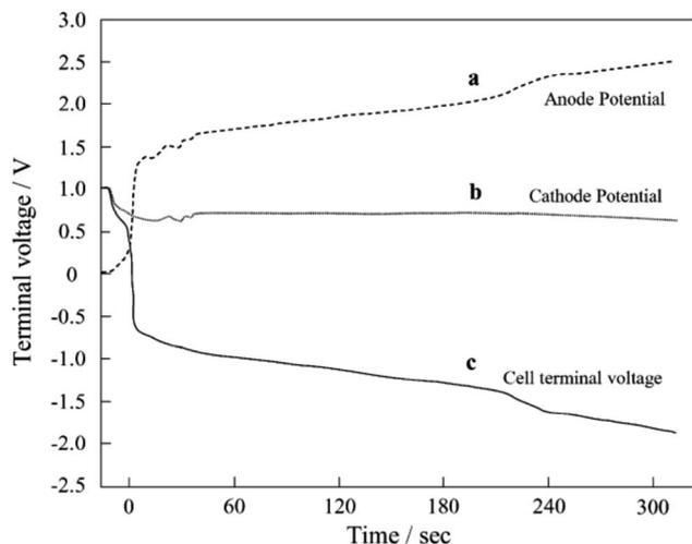
Fig. 2 (a) Anode potential, (b) cathode potential, and (c) cell voltage versus time curves during cell reversal. Reproduced with permission.<sup>19</sup> Copyright 2004, Elsevier.
