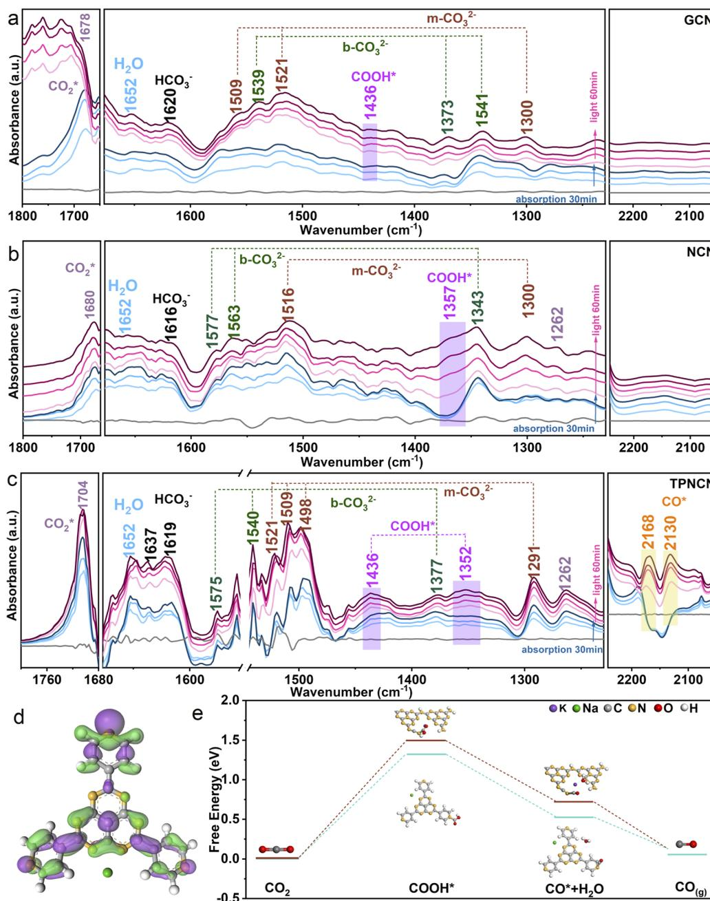
Fig. 4 *In situ* ATR-FTIR spectra of (a) GCN, (b) NCN and (c) TPNCN. (d) Charge density difference of TPHAP. Green and purple regions represent electron depletion and accumulation, respectively. (e) Calculated free energy diagram for the reaction pathways of CO<sub>2</sub> photoreduction for TPHAP and NCN.
