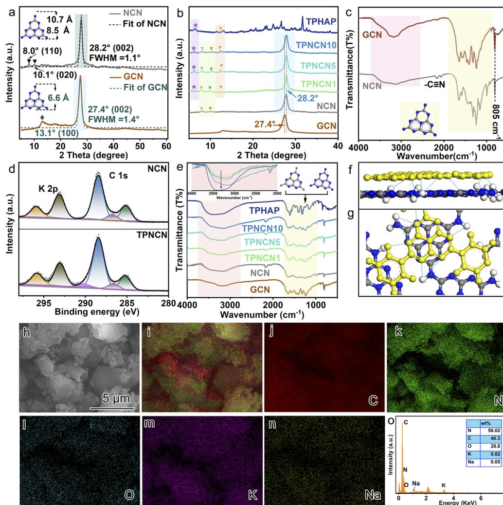
Fig. 1 X-ray diffraction (XRD) patterns of (a) GCN, NCN and (b) TPNCN $m$ . (c) Fourier transform infrared spectroscopy (FTIR) spectra of GCN and NCN. (d) C 1s and K 2p X-ray photoelectron spectroscopy (XPS) spectra of NCN and TPNCN. (e) FTIR spectra of TPNCN $m$ . Schematic illustration for TPNCN $m$  in (f) horizontal and (g) vertical directions. (h) SEM image and SEM-mapping scan images of (j) C, (k) N, (i) O, (m) K, and (n) Na of TPNCN. (o) The mass percentage of all elements.
