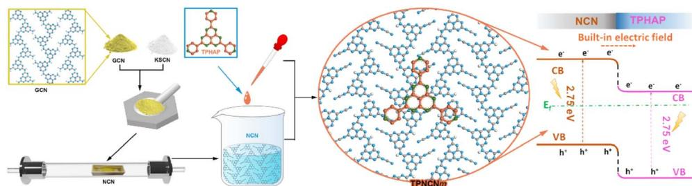
Scheme 1 Schemed fabrication process of the TPNCN photocatalyst.
