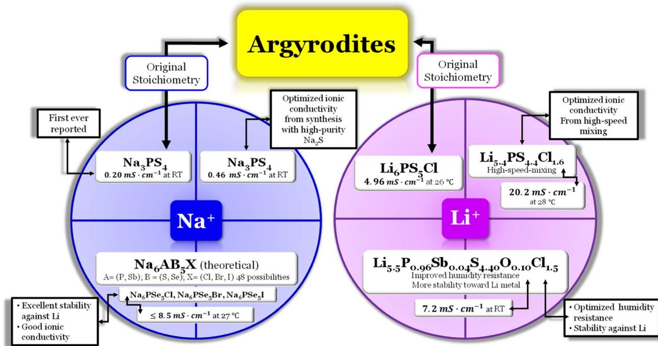
Fig. 6 Argyrodite summary scheme,  $\text{Li}_6\text{PS}_5\text{Cl}$ ,<sup>14</sup>  $\text{Li}_{5.4}\text{PS}_{4.4}\text{Cl}_{1.6}$ ,<sup>30</sup>  $\text{Li}_{5.5}\text{P}_{0.96}\text{Sb}_{0.04}\text{S}_{4.40}\text{O}_{0.10}\text{Cl}_{1.5}$ ,<sup>83</sup>  $\text{Na}_3\text{PS}_4$ ,<sup>84,85</sup> and  $\text{Na}_6\text{AB}_5\text{X}$ , A = (P, Sb), B = (S, Se), and X = (Cl, Br, I).<sup>86</sup>
