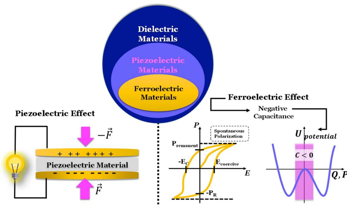
Fig. 9 Dielectric, piezoelectric, and ferroelectric materials and devices. Force  $\vec{F}$ , polarization  $P$ , capacity  $Q$ , electric field  $E$ , potential energy  $U$ , and capacitance  $C$ , remanent polarization  $P_{\text{remnant}}$ , and coercive electric field  $E_{\text{coercive}}$ .
