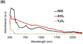
Fig. 4 UV-visible absorption spectra of (A) AQ, ORG, SG and the commercial NiO-YSZ and (B) reference materials NiO, Y2O3 and ZrO2.
