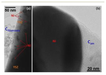
Fig. 8 TEM images of carbon deposits on commercial Ni-YSZ: (a) region revealing the presence of filamentous carbon (Cfilaments) near a group of Ni particles supported on YSZ; (b) a thick amorphous carbon (C<sub>am</sub>) layer partially covers a large Ni particle.
