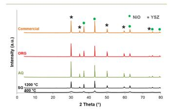
Fig. 3 X-ray diffraction patterns of SG (calcined at 600 and 1200  $^{\circ}$ C for 5 h) and AQ, ORG and the NiO-YSZ commercial samples calcined at 1200  $^{\circ}$ C for 5 h (JCPDF files: NiO: 01-089-5881; YSZ: 01-070-4431).
