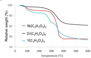
Fig. 1 TG curves of the (A) AQ, ORG and SG precursors and (B)  $Ni^{2+}$ ,  $Zr^{4+}$  and  $Y^{3+}$  propionates.
