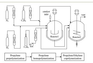
Fig. 1 Flow chart of the experimental device and polymerization procedures
