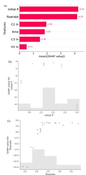
**Fig. 8** (a) Mean absolute SHAP values of process conditions in XGB predicting the rubber phase content; (b) SHAP value for the initial P vs. initial P; (c) SHAP value for the flowrate vs. flowrate.
