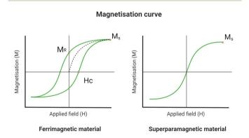
Fig. 2 Magnetisation curve and hysteresis loop of a ferromagnetic and a superparamagnetic material. The curves show the magnetisation saturation (MS), the retentivity (HR) and the coercitivity (HC) (created with BioRender.com).
