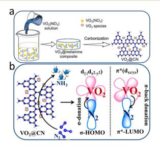
Fig. 1 (a) Schematic representation of the synthesis of VO<sub>2</sub>@CN; (b) orbital interaction between N2 and the VO2 centre of the catalyst, responsible for  $N_2$  reduction to  $NH_3$  (NRR).
