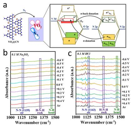
Fig. 5 (a) Orbital interaction between the VO<sub>2</sub> part of VO<sub>2</sub>@CN and N<sub>2</sub> in terms of a molecular orbital diagram; unprocessed in situ ATR-FTIR spectra of the catalyst at different working potentials under N2- and Ar-purged conditions in (b) 0.1 M Na2SO4 and (c) 0.1 M HCl, respectively.
