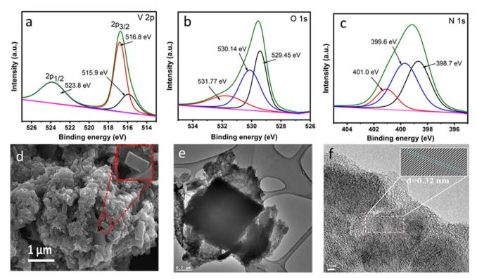
Fig. 3 XPS spectra of VO<sub>2</sub>@CN: (a) V 2p, (b) O 1s and (c) N 1s. (d) FESEM image of VO<sub>2</sub>@CN indicating the presence of blocks of VO<sub>2</sub> encapsulated in crumpled N-doped C layers. TEM and HRTEM images of VO2@CN are presented as (e) and (f), respectively.
