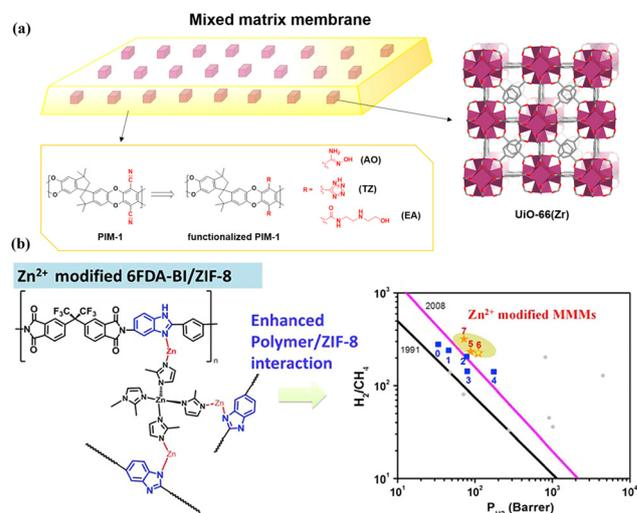
**Fig. 14** (a) Combination of UiO-66(Zr) fillers and PIM-1 functionalized with AO, TZ and EA. Reproduced with authorisation from ref. 94 and copyright 2021 by American Chemical Society. (b) Metal-modified 6FDA-BI/ZIF-8 MMMs and separation performance comparison. Reproduced with authorisation from ref. 95 and copyright 2022 by Elsevier.
