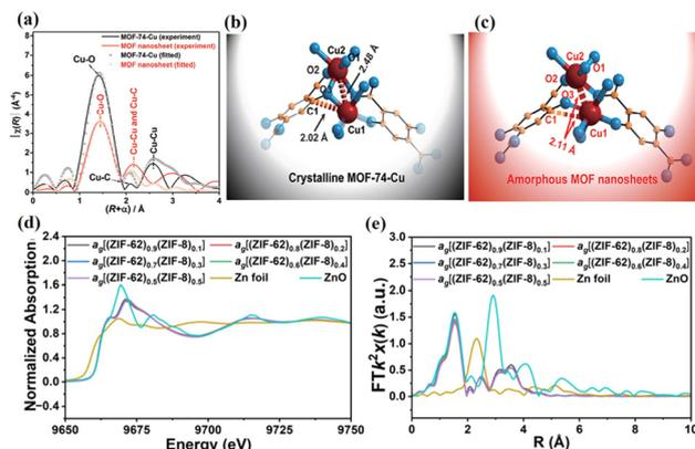
**Fig. 4** (a) EXAFS spectra of MOF crystals and nanosheets. Suggested structures of (b) MOF crystals and (c) nanosheets deduced from the analysis of EXAFS. Reproduced with authorisation from ref. 54 and copyright 2021 by The Royal Society of Chemistry. (d) Normalized XANES spectra and (e) EXAFS R-plots of MOF CGC membranes. Reproduced with authorisation from ref. 45 and copyright 2023 by Wiley-VCH GmbH.
