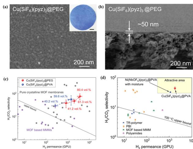
**Fig. 16** (a and b) Surface and cross-section SEM images of Cu(SiF<sub>6</sub>)(pyz)<sub>3</sub>@PEG MMM. (c) Performance comparison of MMMs with different MOF loadings for H<sub>2</sub>/CO<sub>2</sub> separation. (d) Performance comparison of Cu(SiF<sub>6</sub>)(pyz)<sub>3</sub>@PVA MMMs and Ni(NbOF<sub>5</sub>)(pyz)<sub>3</sub>@PVA MMMs with other membranes for H<sub>2</sub>/CO<sub>2</sub> separation. Reproduced with authorisation from ref. 14 and copyright 2023 by AAAS Publishing.
