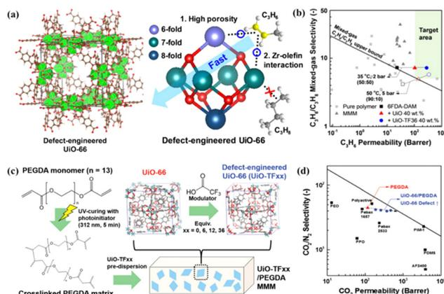
**Fig. 12** Schematic illustration and separation performance comparison. (a and b) Defect-engineered UiO-66/6FDA-DAM MMMs. Reproduced with authorisation from ref. 85 and copyright 2021 by Wiley-VCH GmbH. (c and d) Defect-engineered UiO-66/PEGDA MMMs. Reproduced with authorisation from ref. 86 and copyright 2021 by Wiley-VCH GmbH.
