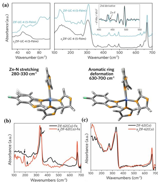
**Fig. 7** (a) Structure comparison of MOF crystals and glass by THz/far-IR and the modes of ZnInM35-Fblm tetrahedra and aromatic rings utilized in DFT calculations. Reproduced with authorisation from ref. 65 and copyright 2020 by American Chemical Society. THz/Far-IR spectra of the vitrification for (b) ZIF-62(Co)-Fe and (c) ZIF-62(Co). Reproduced with authorisation from ref. 66 and copyright 2022 by Wiley-VCH GmbH.
