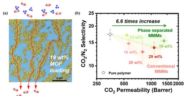
**Fig. 15** (a) TEM image of phase-separated MMMs with 19 wt% UiO-66-NH<sub>2</sub> loading. (b) CO<sub>2</sub>/N<sub>2</sub> separation performance of phase-separated and conventional MMMs with various MOF loadings. Reproduced with authorisation from ref. 18 and copyright 2023 by AAAS Publishing.
