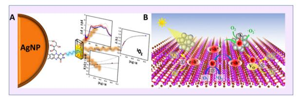
Fig. 15 Schematic representation of singlet oxygen generation from silver nanoparticles. (A) Pectin-stabilized Ag NP. Reproduced with permission.<sup>76</sup> Copyright 2016, American Chemical Society. (B) Defect-free Au NP from FL-BiOBr-NS for enhanced SOG. Reproduced with permission. 77 Copyright 2022, American Chemical Society.
