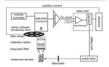
Fig. 5 Schematic diagram of the time- and wavelength-resolved  $^1\mathrm{O}_2$  luminescence detection system. $^{20}$
