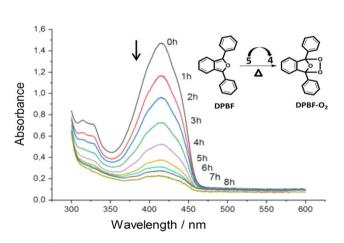
Fig. 10  $\,^{1}\mathrm{O}_{2}$  produced by thermolyzing M-EPO reacts with DPBF. Reproduced with permission.  $^{46}$  Copyright 2020, American Chemical Society.
