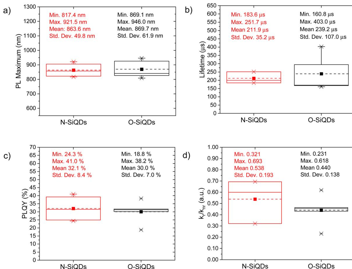
**Fig. 2** Boxplots comparing the (a) PL max, (b) mean PL lifetime, (c) PLQY, and (d)  $k_r/k_{nr}$  of the as-produced N-SiQDs and O-SiQDs. Mean and median of the distributions are represented by dash and solid lines in the boxes, respectively.
