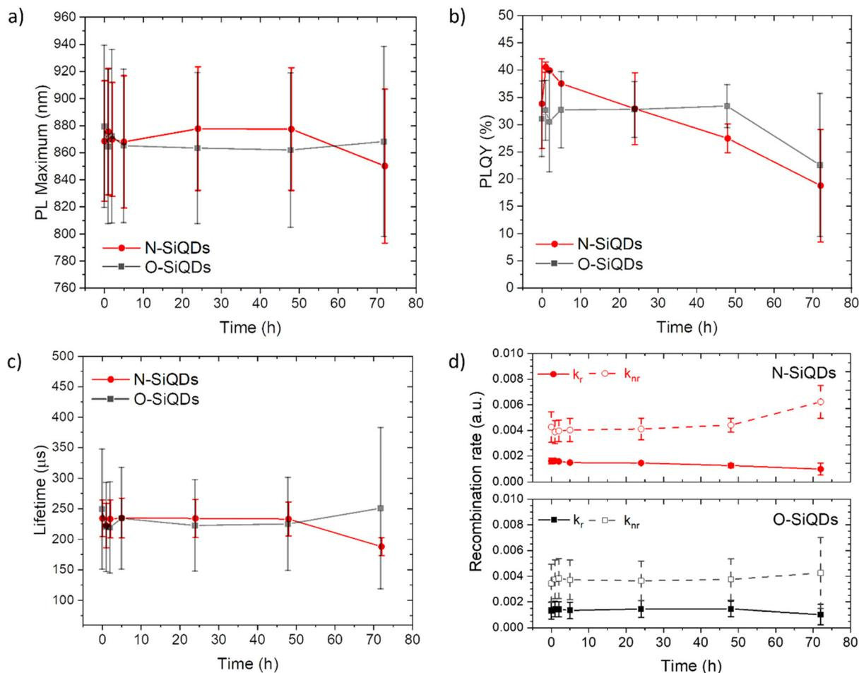
**Fig. 3** A summary of the optical properties of N-SiQDs (red circles) and O-SiQDs (black squares). (a) PL maxima, (b) PLQY, (c) PL lifetime, and (d) recombination rate ratio as a function of time over a period of 72 h of UV irradiation. Error bars represent the 95% limit of measurement. Representative PL and UV-vis absorption spectra of each sample are plotted in Fig. S3, S4 and summarized in Tables S2, S3.†
