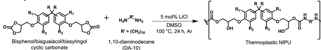
Scheme 1 Synthesis of (a) BGF/BSF using guaiacol/syringol and vanillyl/syringyl alcohol, (b) BGA/BSA using guaiacol/syringol and acetone, (c) diglycidyl ether of bisguaiaicol/bisyringol from respective bisguaiaicol/bisyringol and epichlorohydrin, (d) bisguaiaicol/bisyringol cyclic carbonate from respective diglycidyl ether and CO 2 , and (e) NIPU using respective bisguaiaicol/bisyringol cyclic carbonate and 1,10-diaminodecane (DA-10).
