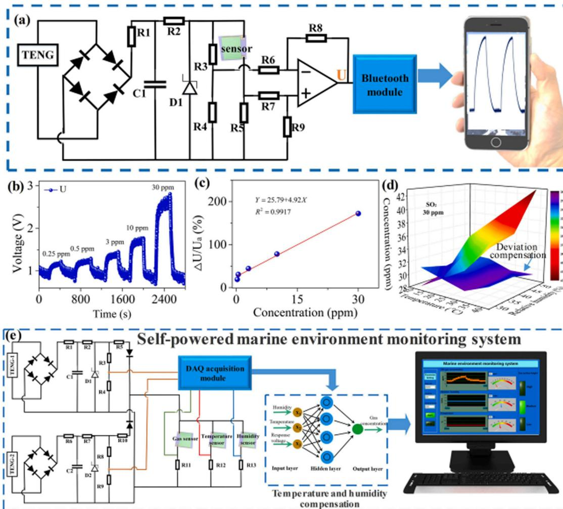
Fig. 3 (a) The wireless sensor detection circuit driven by the liquid–solid TENG. (b) The voltage values of  $U$  and (c) the voltage response ( $\Delta U/U_a$ ) at different  $\text{SO}_2$  concentrations. (d) Comparison of sensor errors caused by temperature and humidity before and after correction. (e) The self-powered marine environment monitoring system. Reproduced from ref. 48 with permission from Elsevier, copyright 2022.
