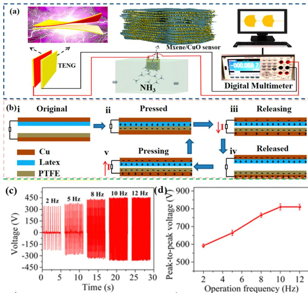
Fig. 5 (a) Schematic illustration of a self-powered NH<sub>3</sub> sensor driven by a TENG. (b) The working mechanism of the TENG. (c) The open-circuit voltage of the TENG at different operating frequencies. (d) Variation trend of output voltage at different operating frequencies. The voltage/current variation. Reproduced from ref. 44 with permission from ACS Publications, copyright 2021.
