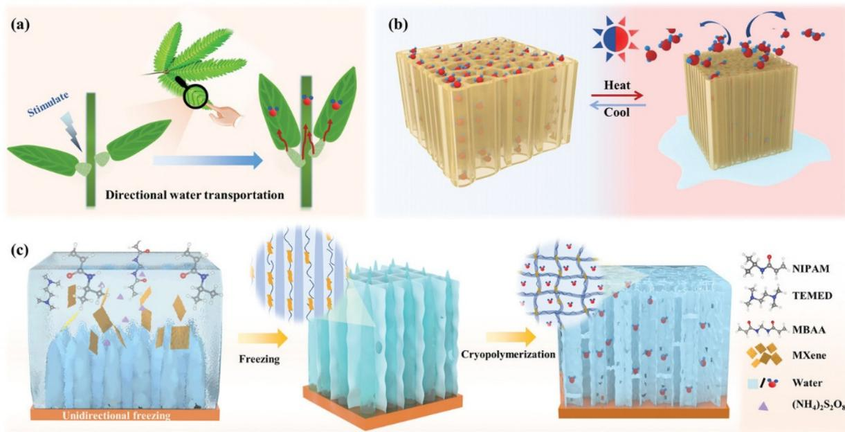
**Fig. 3** Diagram (a) illustrates the closure of a leaf induced by the stimulation and contraction of the mimosa leaf pulvinus. In diagram (b), the process of deformation for a hydrogel actuator with rapid deformation is depicted. Lastly, diagram (c) provides a schematic representation of the synthesis process of the hydrogel, reprinted with permission from ref. 38, copyright reserved Wiley 2023.
