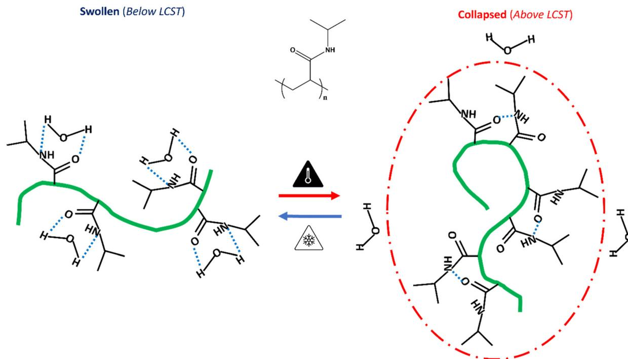
**Fig. 2** Schematic representation of water swelling and de-swelling mechanisms of PNIPAM chains, induced by lower critical solution temperature (LCST) temperature changes, and hydrogen bonding formations.
