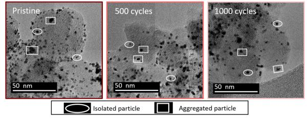
Fig. 1 Representative TEM images of platinum nanoparticles from a Pt/C 20% TKK at 20 µg cm<sup>-2</sup> loading at different stages of cycling between 1.2 and 0.4 V vs. RHE in 1 M H<sub>2</sub>SO<sub>4</sub> + 0.01 M NaCl. The ellipses highlight some examples of isolated particles and the rectangles show some examples of aggregated particles.
