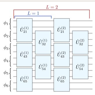
Fig. 1 Circuit structure of the tUPS ansatz.<sup>15</sup> Each qubit encodes the occupation of a spin orbital and the qubits alternate between high- and low-spin orbitals (e.g.,  $\phi_1\phi_1\phi_2\phi_2$ ...).
