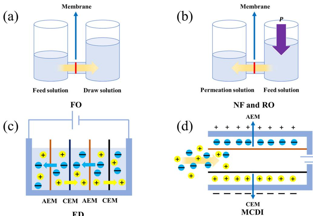
**Fig. 2** Schematic diagram of different driving forces corresponding to technology. (a) FO technology (osmotic pressure driving); (b) NF and RO technology (hydraulic driving); (c) ED technology (electric potential driving); (d) MCDI technology (electric potential driving).
