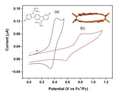
Fig. 7 Cyclic voltammogram of (a) 0.2 mM m-ICz-Br and (b) 0.2 mM (m- $ICz-CN)_2$  in  $CH_2Cl_2/Bu_4NPF_6$  at 298 K; v = 100 mV s<sup>-1</sup>, Pt disk microelectrode.
