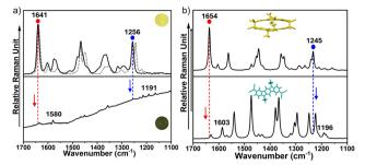
Fig. 13 (a) Top: FT-Raman spectra at  $\lambda_{\rm exc}$  = 1064 nm of the yellow powder of (m-ICz-CN)<sub>2</sub> (black line) and its brominated precursor m-ICz-**Br** (black dots). Bottom: Raman spectrum at  $\lambda_{\rm exc}$  = 785 nm of isolated diradical m-ICz-CN in the solid state at 410 K. (b) Theoretical Raman spectra of  $(m-ICz-CN)_2$  (top) and m-ICz-CN (down) at the M06-2X/6-31G\*\* level
