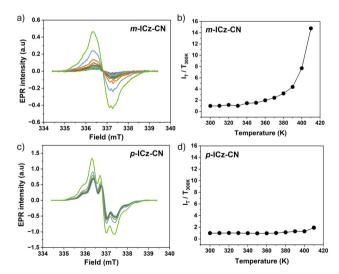
Fig. 12 Variable temperature, cw-EPR spectra of diradical (a) m-ICz-CN and (c) p-ICz-CN generated from dimer cyclophane (m-ICz-CN)2 and (p-ICz-CN)<sub>2</sub>, respectively, in solid state upon gradual temperature elevation from 300 K to 410 K. Experimental conditions: see Fig. 6. T-Dependent relative intensities of EPR signals of diradicals (b) m-ICz-CN and (d) p-ICz-CN measured as polycrystalline powder.
