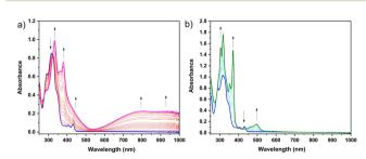
Fig. 10 UV-Vis absorption spectral changes resulting from (a) oxidation of  $(m-ICz-CN)_2$  (blue) to  $[m-ICz-CN]^+$  (purple), and (b) single-step reduction of (m-ICz-CN)<sub>2</sub> (blue) to [m-ICz-CN]<sup>2-</sup> (green). Conditions: in CH<sub>2</sub>Cl<sub>2</sub>/  $Bu_4NPF_6$  at T = 298 K; Pt minigrid in an OTTLE cell.
