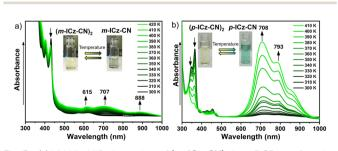
Fig. 5 (a) UV-Vis-NIR absorption of (m-ICz-CN)<sub>2</sub> in o-DCB as a function of temperature. (b) UV-Vis-NIR spectral changes accompanying conversion of dimeric cyclophane (p-ICz-CN)<sub>2</sub> to p-ICz-CN upon heating in o-DCB from 300 to 410 K.
