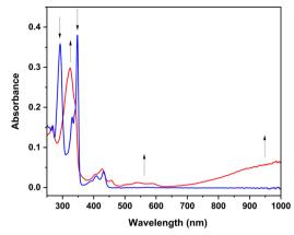
Fig. 9 UV-Vis absorption spectral changes resulting from oxidation of m-**ICz-Br** (blue) to  $[m-ICz-Br]^+$  (red.). Conditions: in  $CH_2Cl_2/Bu_4NPF_6$  at T=298 K; Pt minigrid in an OTTLE cell.
