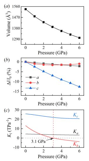
Fig. 2 Evolution of the (a) unit cell volume, (b) relative change rate and (c) linear compressibility of the lattice parameters as a function of pressure. All data were calculated with the DFT-D3(BJ) dispersion correction
