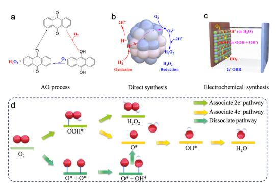
Fig. 1 Illustration of hydrogen peroxide production via (a) traditional anthraquinone process, (b) the direct synthesis, and (c) electrochemical twoelectron oxygen reduction reaction. (d) Illustration of the proposed ORR process.
