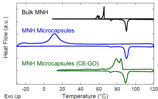
**Fig. 4** Offset DSC data for bulk MNH (black), MNH microcapsules (blue), and MNH microcapsules with C6-GO nanosheets (green). On heating of the bulk sample, melting is observed at ~81 °C, and a lower temperature endotherm is observed at 72 °C, reported to correspond with a solid–solid transition.<sup>32,33</sup>
