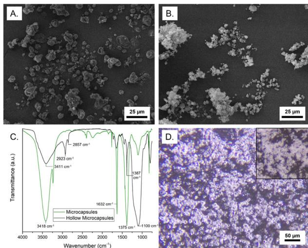
**Fig. 3** SEM images of MNH microcapsules (A) before and (B) after core extraction; (C) FTIR spectra of MNH microcapsules (green) and hollow shells (black); (D) optical microscopy images of MNH microcapsules after heating to 100 °C for 10 min with inset depicting microcapsules at room temperature.
