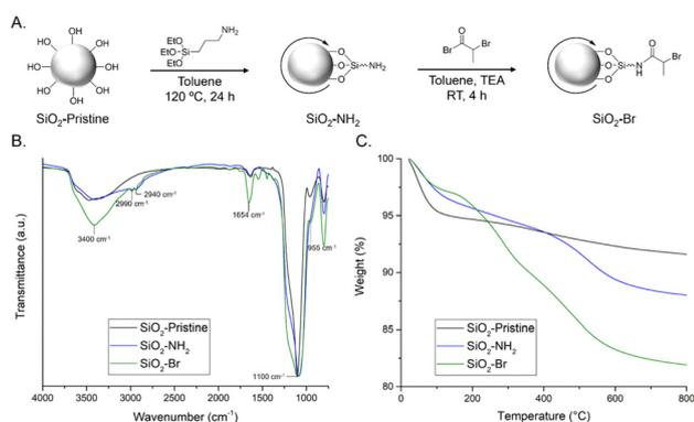
Fig. 2 (A) Schematic of two-step synthesis of SiO<sub>2</sub>-Br from pristine SiO<sub>2</sub>; (B) normalized FTIR spectra; and (C) TGA weight loss profiles of SiO<sub>2</sub>-pristine, SiO<sub>2</sub>-NH<sub>2</sub>, and SiO<sub>2</sub>-Br particles.
