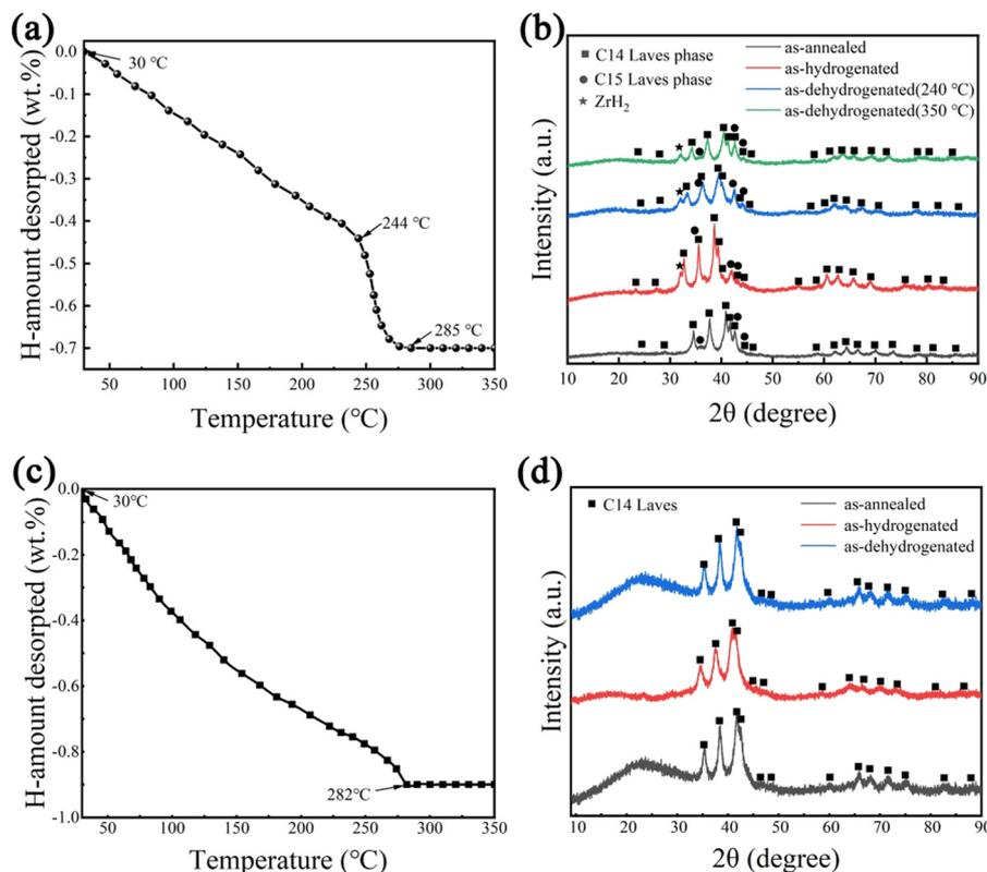
Fig. 7 TPD profile of (a)  $Zr_2MgV_2CrNi$  and (c)  $Zr_2MgVFeCrNi$  high-entropy alloys at a heating rate of  $5\text{ }^\circ\text{C min}^{-1}$ , as well as their XRD patterns for (b)  $Zr_2MgV_2CrNi$  and (d)  $Zr_2MgVFeCrNi$  high-entropy alloys at different states.
