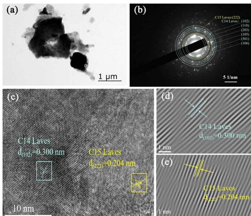
Fig. 4 Microstructural characterization of the  $Zr_2MgV_2CrNi$  sample: (a) TEM image, and (b) corresponding SAED patterns; (c) HRTEM image and the corresponding IFFT images (d) and (e) of C14 and C15 Laves phases.
