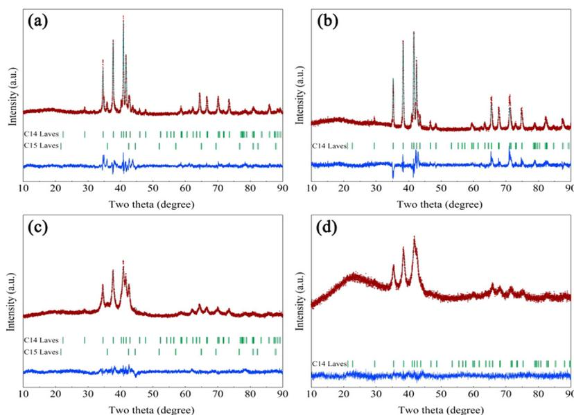
Fig. 1 Rietveld refinements of the XRD patterns for (a) Zr<sub>2</sub>V<sub>2</sub>CrNi, (b) Zr<sub>2</sub>VFeCrNi, (c) Zr<sub>2</sub>MgV<sub>2</sub>CrNi and (d) Zr<sub>2</sub>MgVFeCrNi high-entropy alloys.
