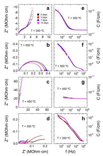
Fig. 2 Time evolution of (a)-(d) Nyquist plots and (e)-(h) capacitance versus frequency response of samples sintered under different conditions: (a), (b), (e) and (f) flash-sintered from micropowder; (c) and (g) conventionally-sintered from nanopowder; (d) and (h) flash-sintered from nanopowder. Samples were flash-sintered at 150 V cm<sup>-1</sup> and 15 mA mm<sup>-2</sup> with a dwell time of 10 min.
