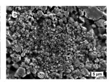
Fig. 4 SEM micrographs of samples sintered under different conditions: (a) flash-sintered sample from micropowder at 150 V cm<sup>-1</sup> and 15 mA mm<sup>-2</sup>; (b) conventionally-sintered sample from nanopowder; (c) flash-sintered sample from nanopowder at 150 V cm<sup>-1</sup> and 15 mA mm<sup>-2</sup>.
