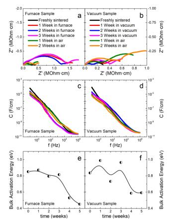
Fig. 6 Time evolution of (a) and (b) Nyquist plots, (c) and (d) capacitance versus frequency response, and (e) and (f) activation energy for bulk conduction of a CCFS sample under a quadratic current profile. The sample is cut in two halves after sintering; one is kept in vacuum and the other in a furnace at 800 °C for three weeks. After that, both halves are stored in ambient atmosphere and measured at one-week intervals for two weeks. Measurements were performed at 350 °C
