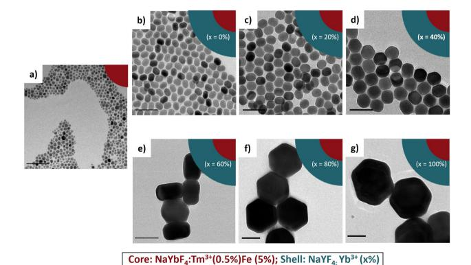
Fig. 1 TEM images of core and core@shell structures using different Yb<sup>3+</sup> concentrations during shell growth. (a) NaYbF<sub>4</sub>:Tm(0.5%) Fe(5%) core and (b)-(g) NaYbF<sub>4</sub>:Tm(0.5%) Fe(5%)@NaYF<sub>4</sub>:Yb(x%)-core@shell where x = 0%, 20%, 40%, 60%, 80%, and 100%. Size histograms are shown in Fig. S1 (ESI†). All scale bars show 100 nm.
