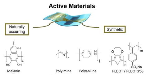
Fig. 5 Bioderived active materials for electronics-Melanine, <sup>43,87</sup> and synthetically derived active materials for electronics-PEDOT: PSS, <sup>31,32,34,48,56,57,59,60,72,75,88–94</sup> polyaniline(PANI), <sup>62,95</sup> polyimine, <sup>25,96</sup> (the structure of melanin has been adapted <sup>97</sup>).
