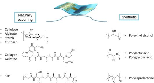
Fig. 4 Bioderived supporting materials for electronics-polysaccharides (cellulose, <sup>48,56-58,65</sup> alginate, <sup>66-70</sup> starch, <sup>34,49</sup> chitosan, <sup>14,34,59-64</sup>), collagen, <sup>71</sup> silk <sup>31,41-43,72</sup> and synthetically derived supporting materials for electronics-polyvinyl alcohol (PVA), <sup>14,16,17,73-75</sup> polyglycolic acid (PGA), polylactic acid (PLA), <sup>19-22,76</sup> polycaprolactone (PCL), <sup>26,27,38,77-79</sup>
