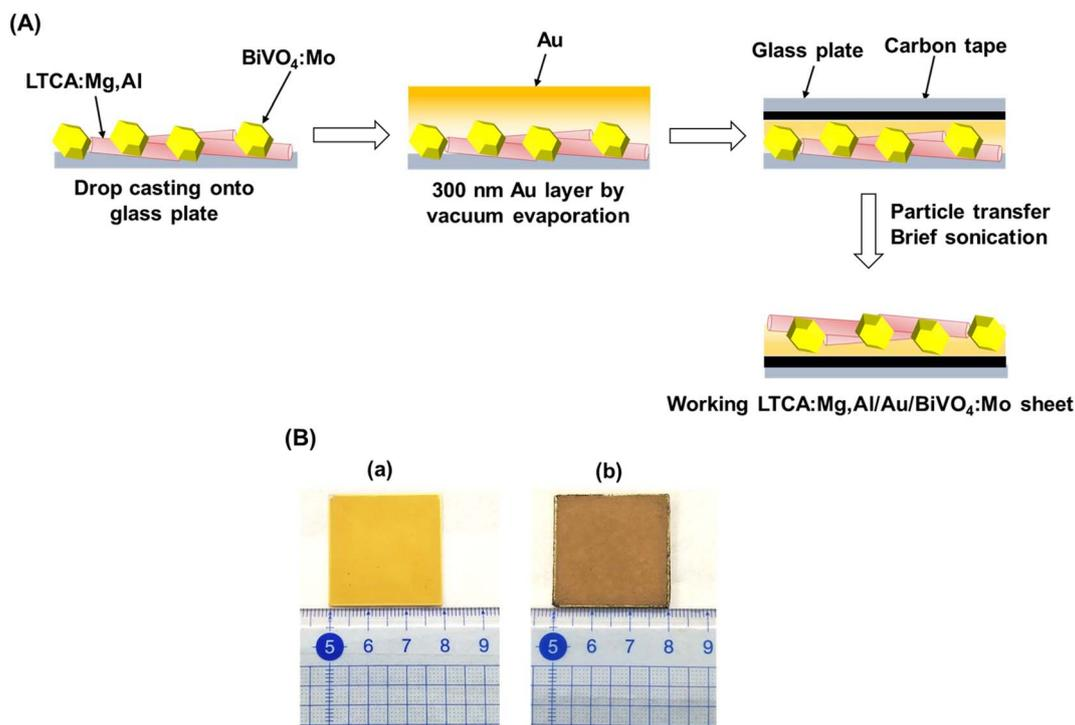
Fig. 4 (A) Schematic illustration of the preparation procedure for photocatalyst sheet composed of LTCA:Mg,Al and  $\text{BiVO}_4\text{:Mo}$ . (B) Photograph of  $3 \times 3 \text{ cm}^2$  LTCA:Mg,Al/Au/ $\text{BiVO}_4\text{:Mo}$  photocatalyst sheet (a) before and (b) after particle transfer. Panel (A) was reproduced from ref. 34 with permission from Elsevier Inc., copyright 2023.
