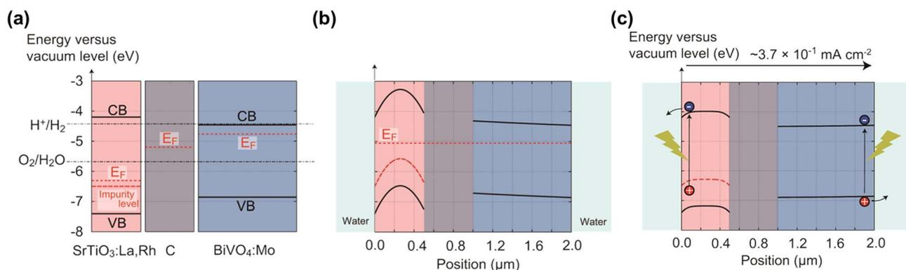
Fig. 3 Band diagrams for SrTiO<sub>3</sub>:La,Rh/C/BiVO<sub>4</sub>:Mo sheet: (a) before contact, (b) under darkness after contact, and (c) under illumination. Reproduced from ref. 28 with permission from American Chemical Society, copyright 2017.
