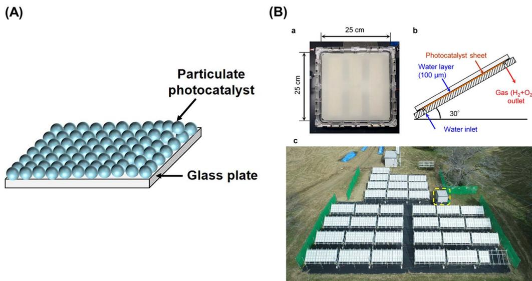
Fig. 2 (A) Schematic diagram of one-step photoexcitation based photocatalyst sheet, (B) 100 m<sup>2</sup>-scale photocatalyst panel reactor: (a) photograph of 625 cm<sup>2</sup> panel reactor unit, (b) schematic side view of panel reactor unit, and (c) top view of 100 m<sup>2</sup> solar hydrogen production system consisting of 1600 panel reactor units. Reproduced from ref. 16 with permission from Springer Nature, copyright 2021.
